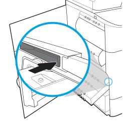
7. Insert the left end of the service fluid container into the alignment track, and then lock the latch that holds the unit in the track.
