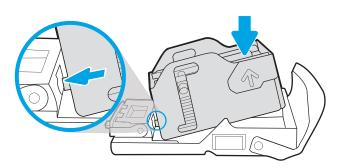
5. Insert the staple cartridge into the stapler and push on the colored handle until it snaps into place.
