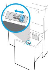
Load paper into the tray. Check the paper to verify the guides lightly touch the stack, but do not bend it.
