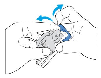
4. Close the lever at the back of the staple cartridge. Be sure that it snaps into place.
