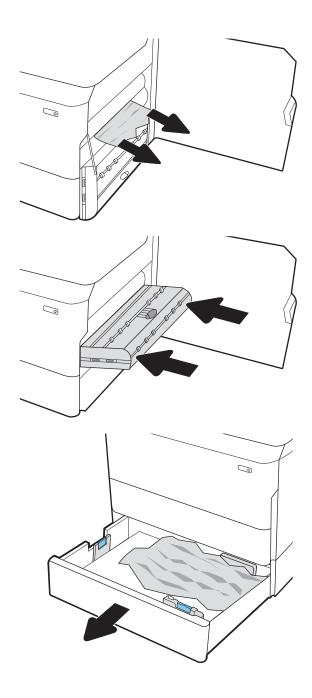
7. Remove the jammed paper from the feed rollers inside the printer. First pull the paper to the left, and then pull it forward to remove it.
