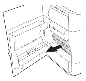
3. On the left side of the service fluid container, release the latch that holds the unit in the alignment track, and then remove the left side of the unit.
