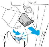
4. Lift up on the small lever at the back of the staple cartridge to separate the staple cartridge from the holder, and then remove any jammed staples.
