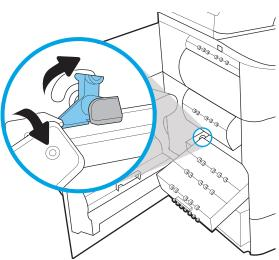
Push the service fluid container into the printer.
