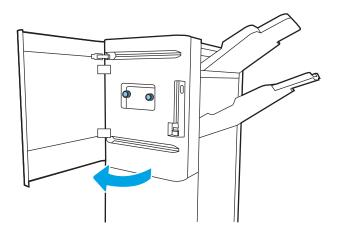
Rotate the green knobs, and then remove any jammed paper.
