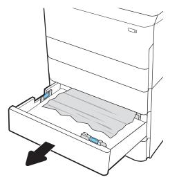
2. Remove the jammed paper from the feed rollers inside the printer. First pull the paper to the left, and then pull it forward to remove it.
