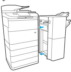
Clear paper jams in the floor standing finisher front door (E77650z+, E77660z+, P77940dn+, P77950dn+, P77960dn+ models only)
