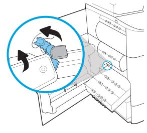
4. Remove the right side from the alignment track, and then remove the unit from the printer. Set the unit aside, upright, on a piece of paper to prevent spills.
