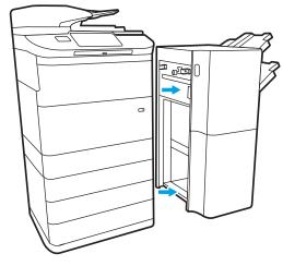
Move the finisher to a position where the finisher rear door is accessible, and then open the finisher rear door.
