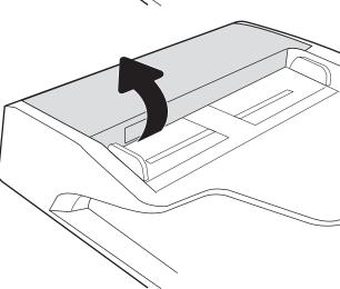
Remove any visible lint or dust from each of the feed rollers and the separation pad using compressed air or a clean lint-free cloth moistened with warm water.
