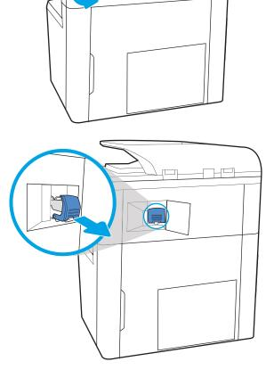
3. Insert the new staple cartridge into the stapler and push on the colored handle until it snaps into place.
