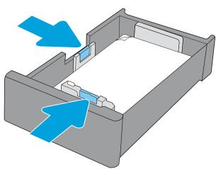
To prevent jams, do not overfill the tray. Be sure that the top of the stack is below the tray full indicator.
