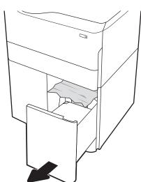
13. Remove the jammed paper from the feed rollers inside the printer. First pull the paper to the left, and then pull it forward to remove it.
