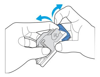
5. Close the lever at the back of the staple cartridge. Be sure that it snaps into place.
