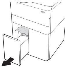
11. Remove the jammed paper from the feed rollers inside the printer. First pull the paper to the left, and then pull it forward to remove it.
