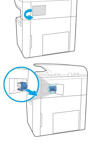
3. Lift up on the small lever at the back of the staple cartridge to separate the staple cartridge from the holder, and then remove any jammed staples.
