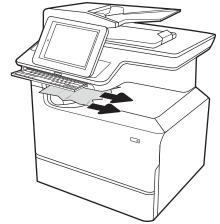
Open the left door. If jammed paper is visible inside the jam-access door, pull it straight out to remove it.
