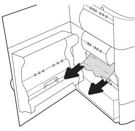
5. If no jammed paper is visible, pull the service fluid container out.
