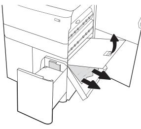
9. Close the jam cassette, and then reinstall it into the printer.
