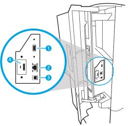
Host USB port for connecting external USB devices
