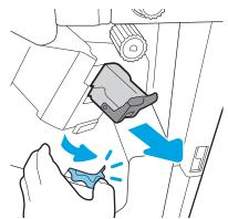
4. Insert the new staple cartridge by holding the green wheel with one hand while pushing the staple cartridge into the slot.
