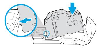
6. Insert the staple cartridge by holding the green wheel with one hand while pushing the staple cartridge into the slot.
