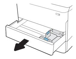
2. Adjust the paper-length and paper-width guides by squeezing the blue adjustment latches and sliding the guides to the size of the paper being used.
