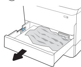
7. Remove the jammed paper from the feed rollers inside the printer. First pull the paper to the left, and then pull it forward to remove it.
